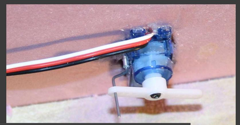
Make U in one end Push piano wire down thru turnout and foam Push tubing up around wire Cut pocket in foam for body Bend wire to form crank
