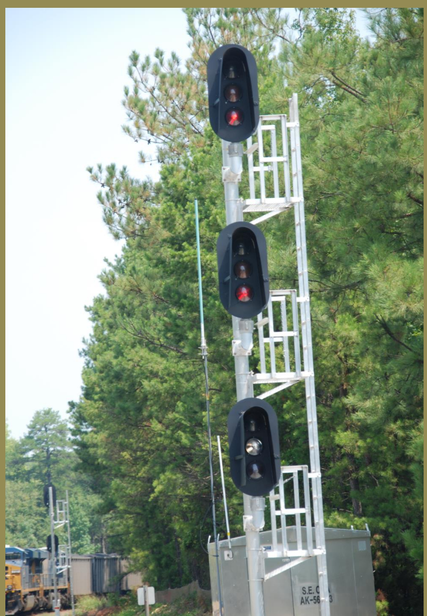
New CSX Color Lights South end Ora Note: Top two G/Y/R, bottom G/Lunar/R
