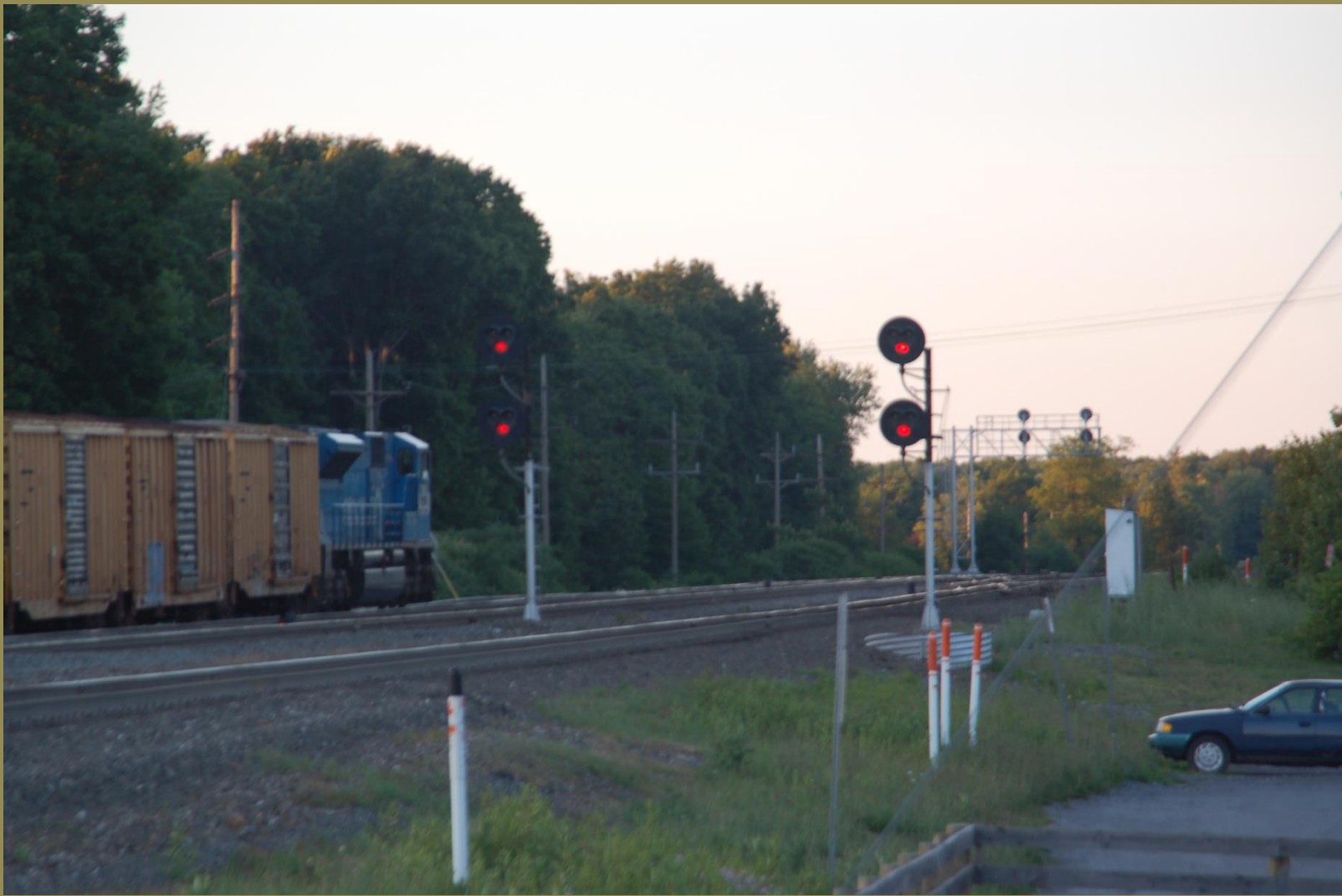
New NS TriLight Signals Cresson, PA, replaced PRR PL's
