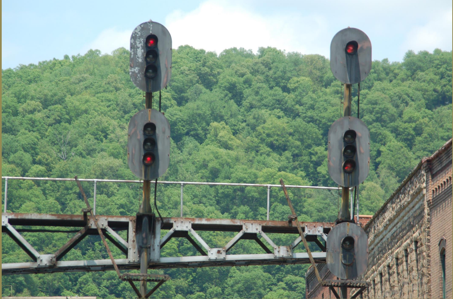
Color Lights on former C&O, Thurmond, WV Note: Red locations > better separation
